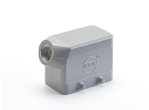
Specifications:10B,Housing type:Surface mounting upper housing,Outgoing method:Side outlet,Locking type:Dual lock,Thread:M20,Housing material:Die casting aluminum,Material:Galvanized iron,Seals:NBR
